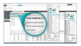
· If you want to assign all data to just one marking material, enable the "Enforce default material" check box and then select your marking system and the corresponding material.
