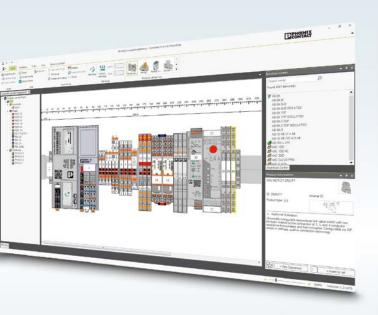
In PROJECT complete, you can replace automatically selected terminal blocks, add accessories, and exchange wire bridges with plug-in bridges. After editing the terminal strip, the changes are exported to EPLAN Electric P8 / EPLAN Pro Panel.
