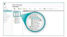
The import configuration files are listed on the "EPLAN Electric P8" tab. This is where the marking systems and marking materials used are assigned to the relevant product order numbers.
